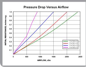
The Camfil Filtra 2000 provides high-efficiency particulate air filtration for critical application processes. With more than double the media of standard HEPA filters, critical airflow and energy savings are always optimized. Available in airflow capacities up to 2400, the Filtra 2000 includes:
